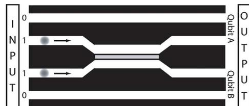
FIG. 1. (Color online) Each qubit is a pair of waveguides. The spatial location of the electron in the waveguides determines the state of the qubit. Here both qubits are in state  $|1\rangle$ . The waveguides representing state  $|1\rangle$  are brought near each other to facilitate the Coulomb interaction of the electrons, effecting a two-qubit unitary transformation.
