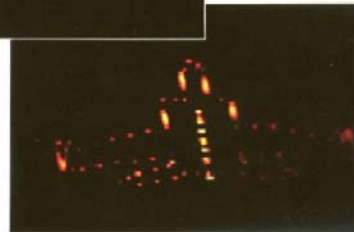
JTFA-Based ISAR Image of a MIG-25
